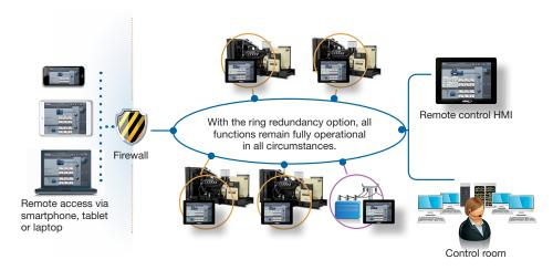
The ring is created by several Ethernet segments and groups together regulation and PLC communications.
